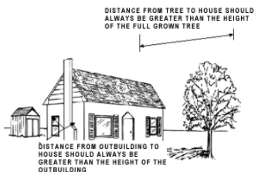
Figure 2. Clearance Around a Building
