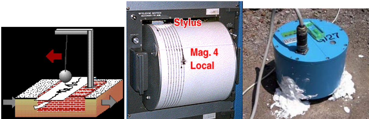
Visual 5.8 - From the left, a schematic depiction of a seismograph; a drum-type seismograph, popular until the early 1990s, and an actual seismometer (right) being installed at a site in Japan. Photo credits: Seismograph drum: USGS; seismometer: http://hakusan.s.kanazawa-u.ac.jp/~yoshizo/elephants/hakusanseis2001.html
