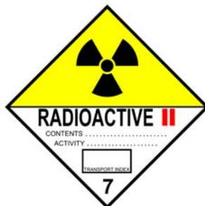
**Radioactive Yellow-II:** medium-level radiation levels detectable outside the package.
